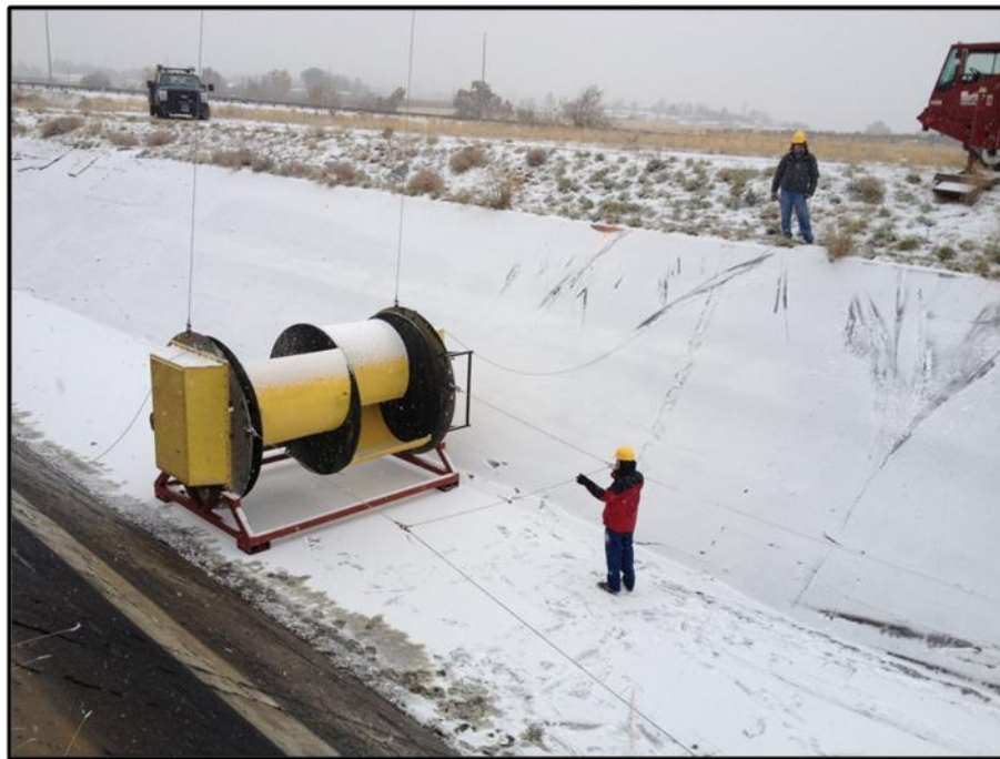
Chief Engineer Jim Styner conducting a dry run test install of the Hydrovolts turbine prototype in Roza canal.
