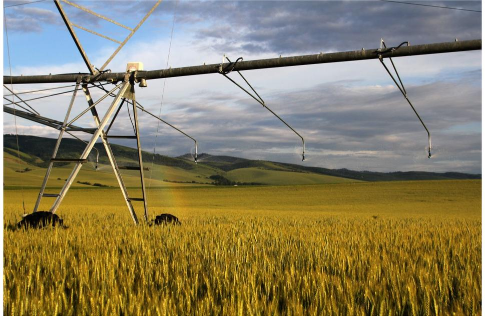
Extension arms called boombacks move water away from the frame of a pivot irrigation system. Photo courtesy of IACO.
